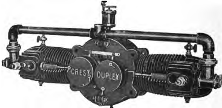
FIG. 233.—"Crest" Double-Opposed Cylinder Gasoline Vehicle Engine, showing radiating ribs for cooling cylinders. The cylinders of this motor are in line, not off-set, as in some makes, the two cranks working on one crank pin. Owing to the method of joining the crank case on its diameter, all the working parts may be readily reached by unscrewing four bolts. Among the special features of this motor are the relief valve, which opens, hence interrupting operation as the wagon coasts down hill, and the automatic cut out for the battery circuit which operates when the engine is at a standstill.
